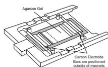
4. Place a SPIFE Blotter C on the gel with the longer edge parallel with gel blocks. Gently blot the entire surface of the gel using slight fingertip pressure on the blotter, and remove the blotter.
